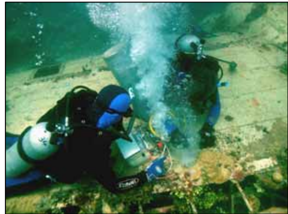
Figure 1 – CoPI Dr Ian MacLeod and July 2006 Earthwatch volunteer Neil Glickstein drilling a hole in the wing of the Emily flying boat in preparation for measuring the corrosion potential of the aluminium. Photo courtesy of Bill Jeffery.
